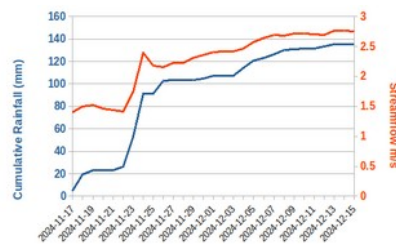
Figure 12: Lambourne - streamflow and cumulative rainfall - Nov-Dec 2024
